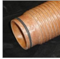
**SP/SPH** joints are 4 threads-per-inch with round form (SP) or buttress (SPH) profiled sealing threads. A secondary seal is provided by an o-ring gasket fitted within a groove in the male end. This exceptionally user friendly connection is used in high pressure applications up to 2,500 psi (17.2 MPa) and temperatures up to 212°F (100°C).
