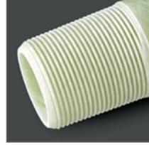
**Precision Ground Thread (PGT)** is produced with numerically controlled grinding equipment and the tolerances provided by PGT require only the use of Teflon base lubricant or proprietary sealant for make-up. The PGT connection is manufactured according to the industry standard EUE 8rd or OD 8rd thread, as is the case for the ACT thread described in the upper left
