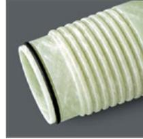
**STAR Super Seal (SS, SS HP)** is a fast, reliable, all-weather and self-restrained mechanical o-ring seal. O-rings are standard Nitrile for normal applications up to 212°F (100°C).
