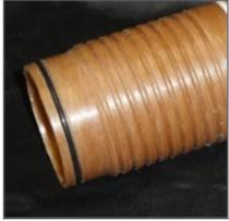
**CEN** is a 4-thread per inch modified ACME thread (non-sealing) joint that seals with an O-ring seal fitted within a groove in the male end. It is used primarily in low pressure flow line or transfer applications in pressures from 500 psi (3.5 MPa) and temperatures up to 212°F (100°C).
