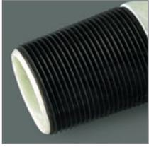
**Advanced Composite Thread (ACT)** connection is manufactured with a special composite consisting of epoxy, graphite, and ceramic. These materials with a Teflon® base lubricant or proprietary sealant, and the consistent tolerances of ACT, provide exceptional sealability to high pressure fluids and gases with excellent make-up and break-out performance. The molded ACT provides higher thread shear and chemical resistance and is preferred over cut or ground fiberglass threads for downhole tubing.
